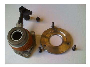
When fitting this solid flywheel replacement kit, the concentric slave cylinder must have the spacers supplied fitted between the cylinder & the gearbox, and the inlet pipe & the gearbox to obtain the correct release point.
