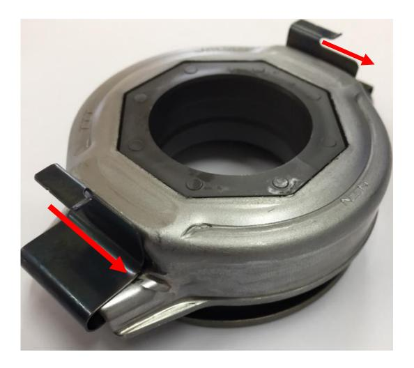
Installing the bearing the incorrect way has been contributed to some recorded cases of shudder in some vehicles.
