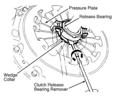
The installation process requires the release bearing to be installed onto the clutch fork. The transmission is then installed and the release lever is to be pulled the opposite direction of its normal operation. The release bearing will then click into the cover assembly.
