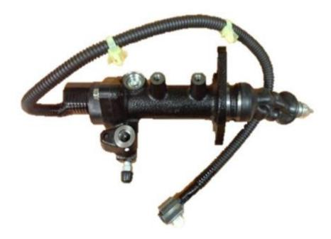
A faulty slave cylinder will impact the functionality of the clutch and may result in premature failure, slip or non release.
